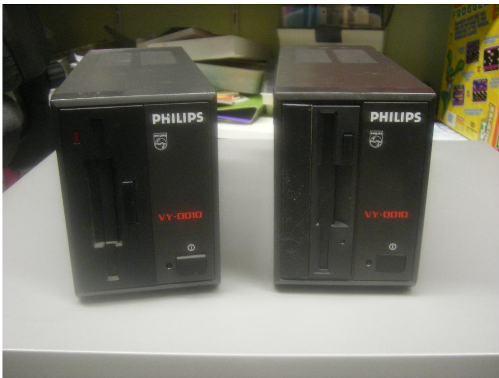
On the left the VY 0010 before the conversion and on the right after the conversion.
