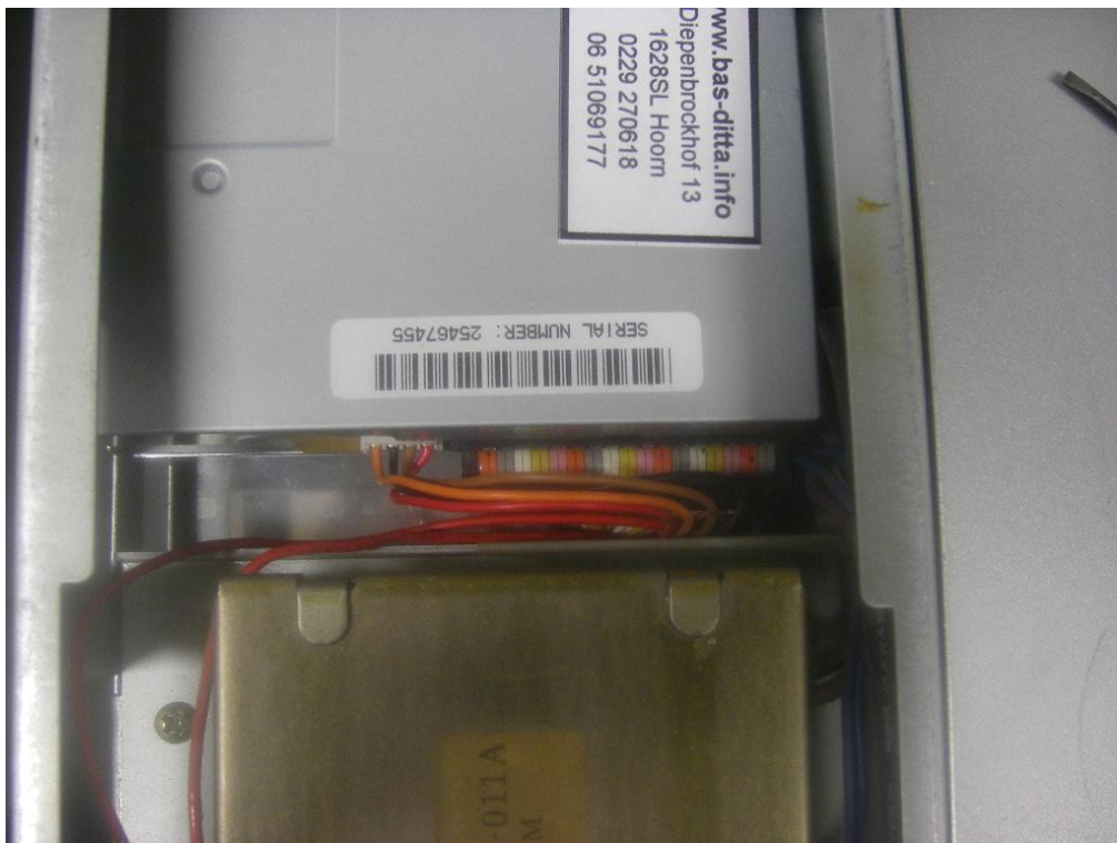
The new double-sided disk drive with connected cables.
