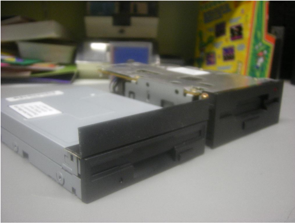
On the left the double-sided disk drive with angle profile, on the right the original single-sided disk drive.
