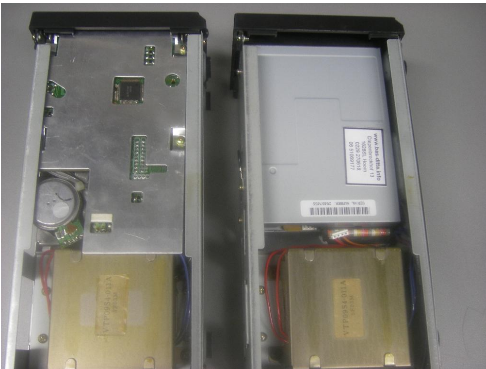
On the left the original single-sided disk drive, on the right the new double-sided disk drive.
