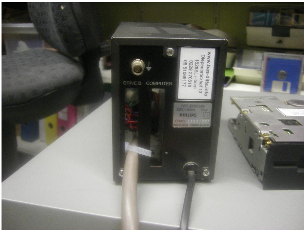
The back of the VY 0010 with a cable tie as strain relief.
