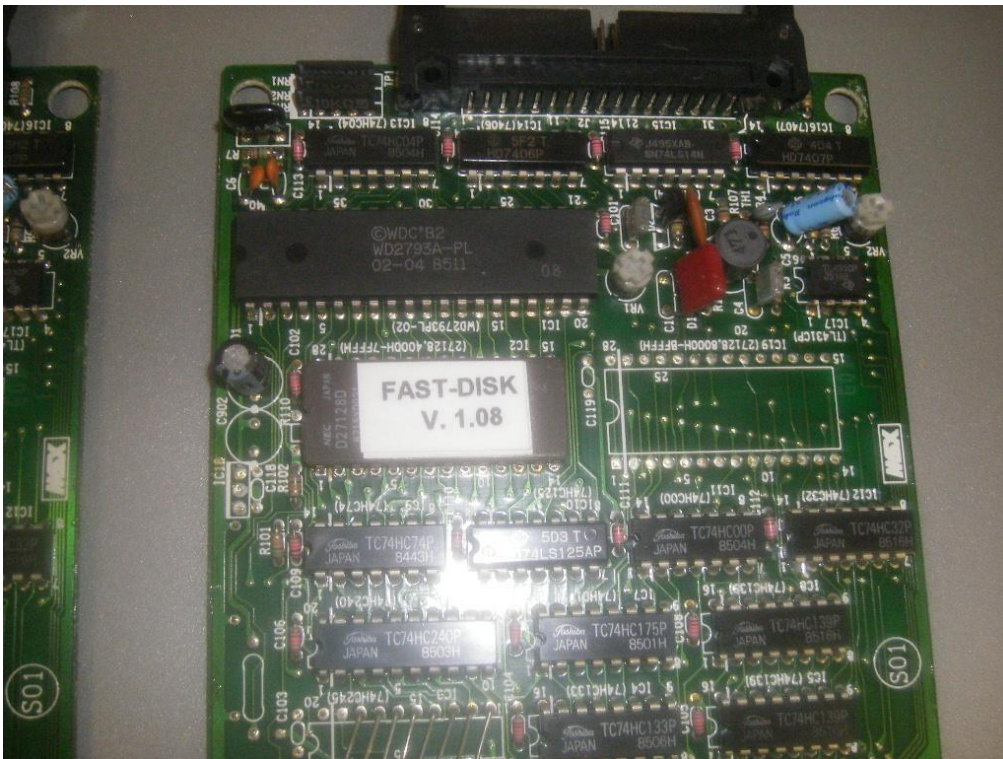
The interface with replacement disk ROM.
